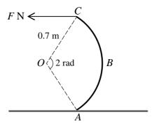
The diagram shows a uniform object ABC of weight 3 N in the form of an arc of a circle with centre O and radius 0.7 m. The angle AOC is 2 radians. The object rests in equilibrium with A on a horizontal surface and C vertically above A. Equilibrium is maintained by a horizontal force of magnitude F N applied at C in the plane of the object. Calculate F.
